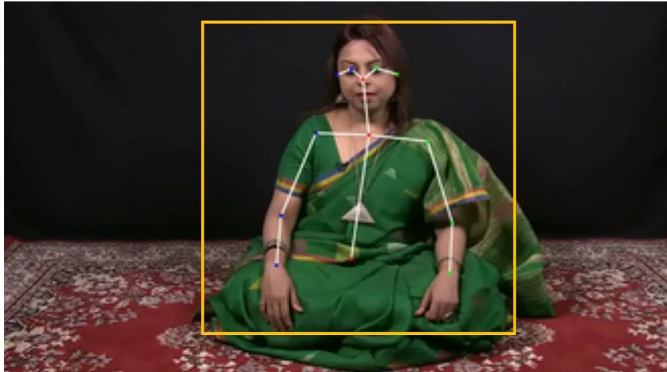
Figure S1: Figure indicates the bounding box over which the movements of the singer is normalized from video data. The box is defined by the most extreme movements of 11 keypoints (eyes, nose, neck, shoulders, mid-hip, elbows and wrists) along the x and y axes. The x coordinates are normalized over the width of the box and the y coordinates are normalized over the height of the box.
